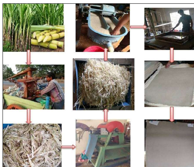
Plate 1. Manufacturing process of handmade paper
