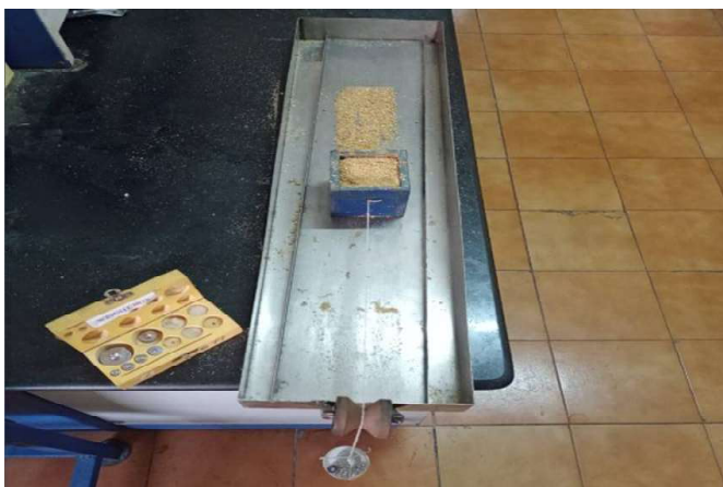
Plate 1. Measurement of static coefficient of friction
