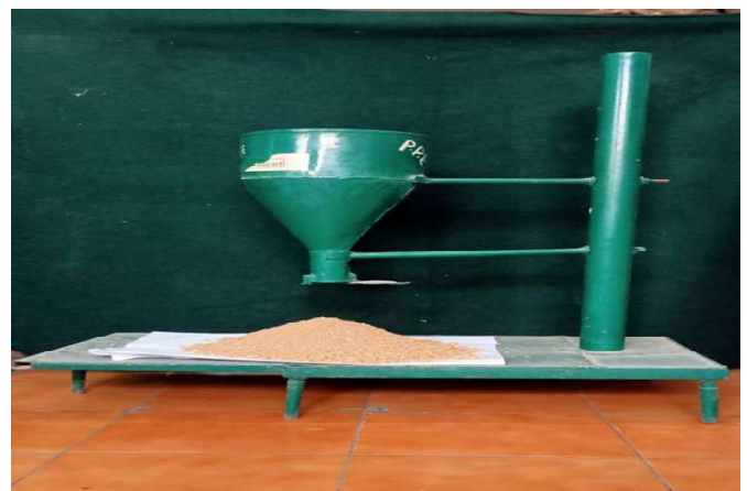
Plate 2. Measurement of angle of repose
